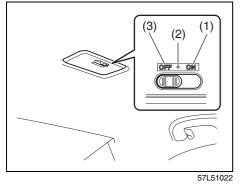
The interior light switch has three positions, which functions as described below.
